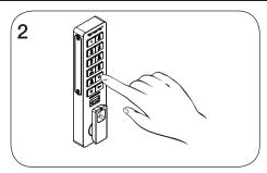
While the LED is on, press C [assigned user code] Om.
