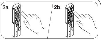
While the LED is on, press C [new 4-7 digit code] Om.
