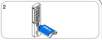
While the LED is on, insert a User Key.
