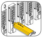
Insert the Programming Key to program each lock to operate with the same user credentials and Manager Keys.
