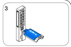
While the LED is on, insert a new User Kev.
