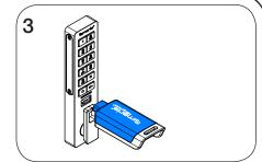
While the LED is on, insert a new User Key.
