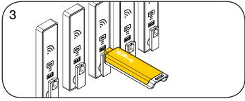
Insert the Programming Key to program each lock to operate with the same user and manager credentials.
