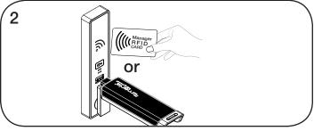
While the LED is on, insert one Manager Key or present one RFID Credential at a time.
