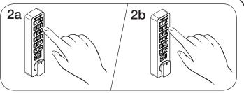
While the LED is on, press C [a new 4-7 digit code] Om.
