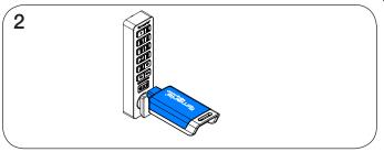
While the LED is on, insert a User Key.
