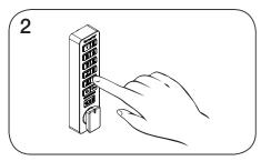
While the LED is on, press C [assigned user code] Om.
