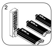
While the LED is flashing, insert one Manager Key at a time.
