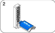
While the LED is on, insert the assigned user Key.
