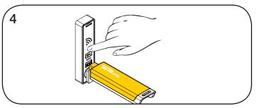
End Express Registration mode:\* Go to any programmed lock. Touch Orm then insert the Programming Key.
