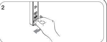
To lock: Close the door then turn the knob to the locked position.
