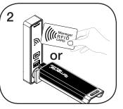
While the LED is flashing, insert a valid Manager Key or present a valid Manager RFID.
