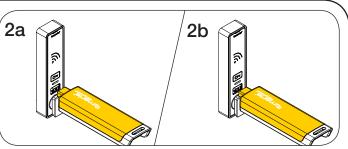
While the LED is flashing, insert the Programming Key.
