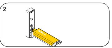
While the LED is flashing, insert the Programming Key. A two-tone beep will be heard and the LED will turn off.
