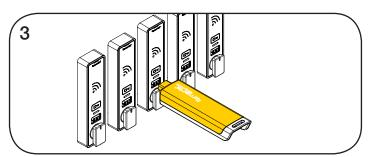
Insert the Programming Key to program each lock to operate with the same user and manager credentials.
