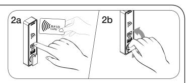
To unlock: Touch 🗁 and present the same User RFID Credential, then turn the knob to the unlocked position. Open the door.
