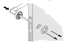
Insert the mechanical door handle keeping it in a horizontal position. For door handles pointing to the right, tighten the rosette towards the left, guide it over the handle holder and engage the bayonet lock. Accordingly, tighten the rosette towards the right for door handles pointing to the left.
