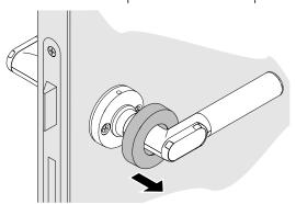
Loosen the mounting screws. Remove the inner electronic door handle from the square pin. Remove the outer electronic door handle from the lock.
