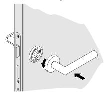
Insert the locking screw from the bottom of the rosette and tighten it.
