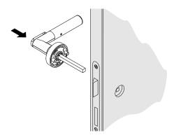
Place the drilling template on the square pin, align horizontally and center punch the hole markings.
