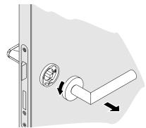
Unscrew the handle holder. Remove the electronic door handle from the lock
