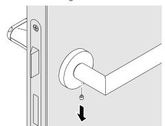
Loosen the bajonet lock. To do this, tighten the rosette to the left for door handles pointing to the right and remove the mechanical door handle from the square pin. Accordingly, tighten the rosette towards the right for door handles pointing to the left.
