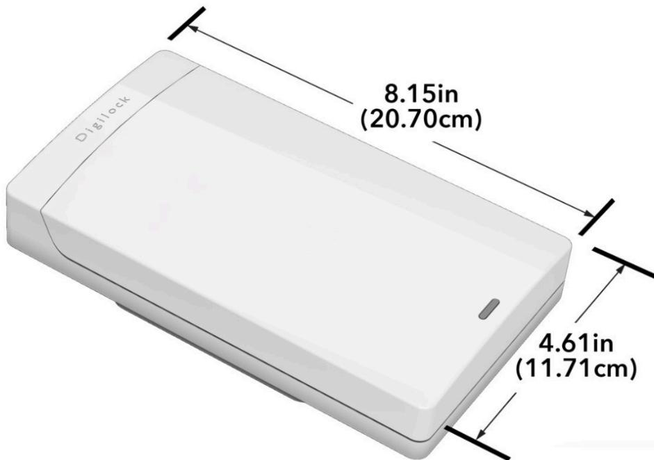
The DG-Gateway sends and receives data streams via the internet router and then transmits information to the locks. Gateways should be installed within a maximum range of 50 feet (approx. 15.25 meters) from the locks. If the building layout allows, they should be mounted within line of sight of the locks. It is recommended to install the DG-Gateway on the ceiling to prevent potential obstacles that could block the signal to the lock.
