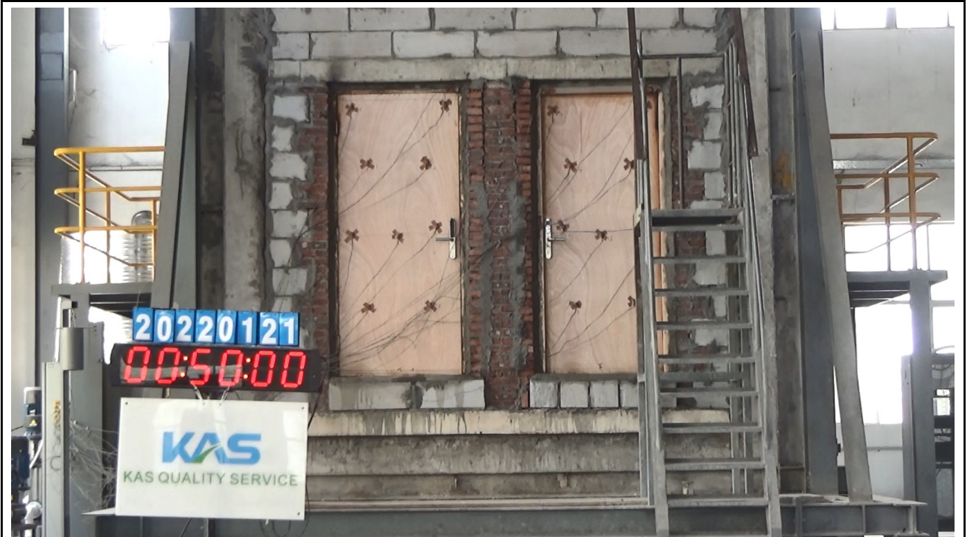
After 50 min (Unexposed Side)
