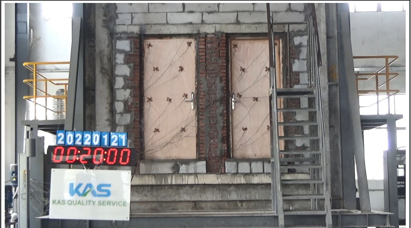
After 20 min (Unexposed Side)
